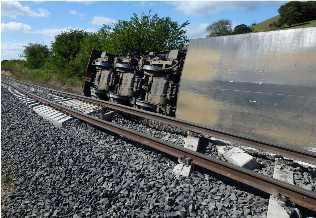
Figure 4: Sleepers pushed into bunches adjacent to locomotive TR10.
