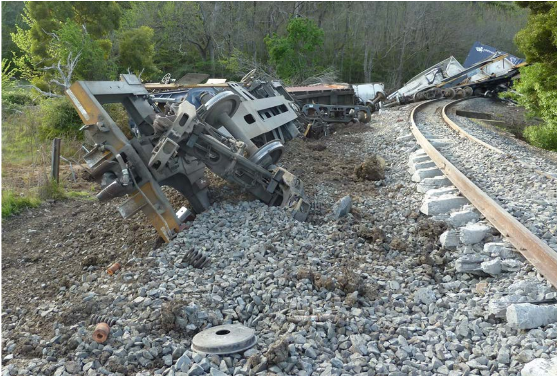
Figure 3: Derailed Wagons on the right hand side of the track and wagons behind stacked on the track.
